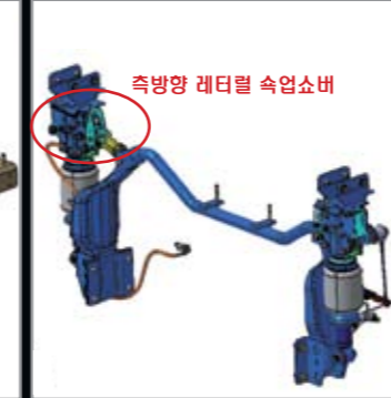
후면 캡 서스펜션 PSD (Position Sensitive Damper)
