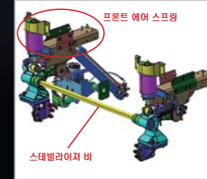
전면 캡 서스펜션 PSD (Position Sensitive Damper)
