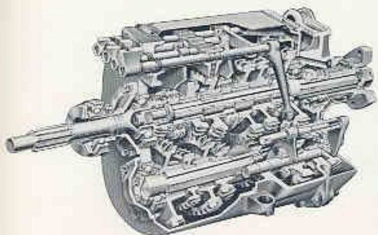
The 5-speed constant-mesh gearbox is a true heavy-duty unit built to withstand the most severe treatment. All gears are of case-hardened nickel-chrome steel, and to ensure silence in operation, helical gears are used for 3rd, 4th and 5th speeds. To improve fuel consumption, or to obtain a higher road speed, a helical-toothed overdrive 6th speed, with a .76 to 1 ratio, can be incorporated at an extra charge. A 50 h.p. low or high-speed power take-off can be fitted on side of box.
