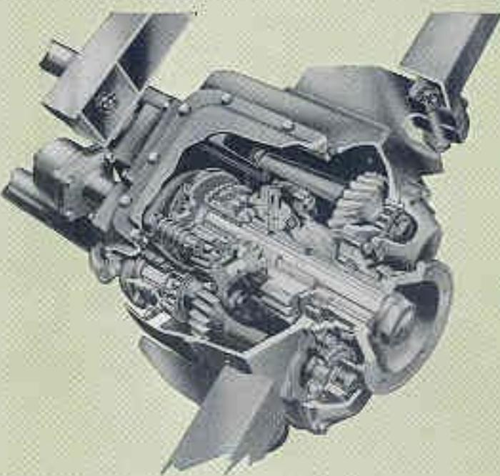
On twin-drive models a relay gearbox is fitted, which divides the drive from the main gearbox into two, thus providing two final-drive shafts. One is coupled direct to the No. 1 axle, while the other passes through the leading axle body via a relay shaft to the second axle. It incorporates a locking differential, controlled from the driver's cab, for use when ground conditions are difficult, e.g., over soft ground or on ice.
