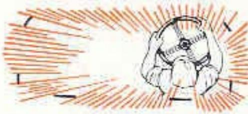
Full curved windscreen with twin wipers, swivelling quarter lights and full-drop winding windows, supplemented by a central rear window, with curved quarter light on each side, ensure perfect all-round visibility. The total glazing area is approximately 3,000 sq. in. (19,355 sq. cm.).
